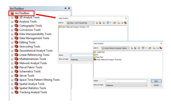
The UNA Toolbox should now appear at the bottom of ArcToolbox, below the 'Tracking Analyst Tools'
